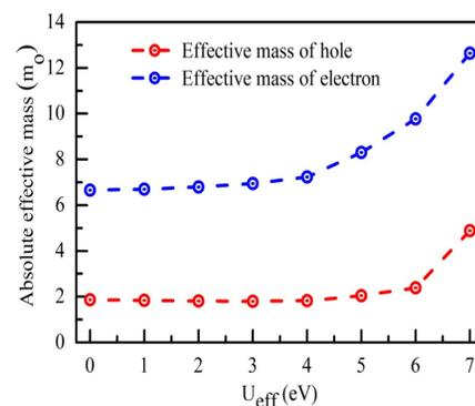
Fig.4 : Variation of the absolute effective masses of holes and electrons in terms of the electron rest mass, m<sub>0</sub> with the increase of U<sub>eff</sub> values.
