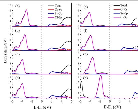
Fig.5 : The calculated total density of states (TDOS) of CsSnCl<sub>3</sub> and the Cs 6s, Sn 5p and Cl 3p orbitals.
