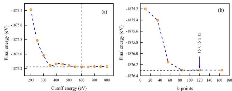
Fig.1 : (a) Plane-wave cutoff energy convergence (b) k-points grid variation for structure optimization of CsSnCl<sub>3</sub>
