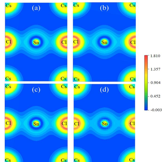
Fig.6 : Electronic charge density along (110) plane of CsSnCl<sub>3</sub> for (a) U<sub>eff</sub> = 0 eV, (b) U<sub>eff</sub> = 3 eV, (c) U<sub>eff</sub> = 6 eV, and (d) U<sub>eff</sub> = 7 eV
