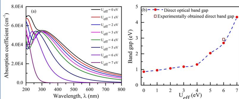
Fig.3 : (a) Absorption coefficient variation as a function of wavelength for various U<sub>eff</sub>. (b) Direct optical band gap as a function U<sub>eff</sub>. For U<sub>eff</sub> = 6 eV the theoretically calculated direct optical band gap matches well with the experimentally obtained direct band gap of 2.98 eV (square marked).
